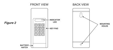
The RF Programmable Keyless Entry System has two programmable codes:
